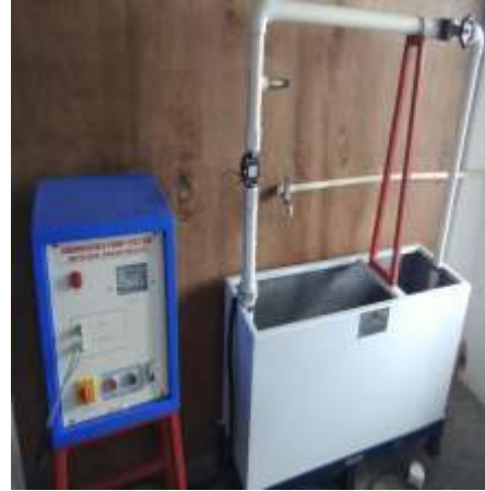
Figure 6 Submersible Pump Apparatus (Hydraulics Laboratory)
