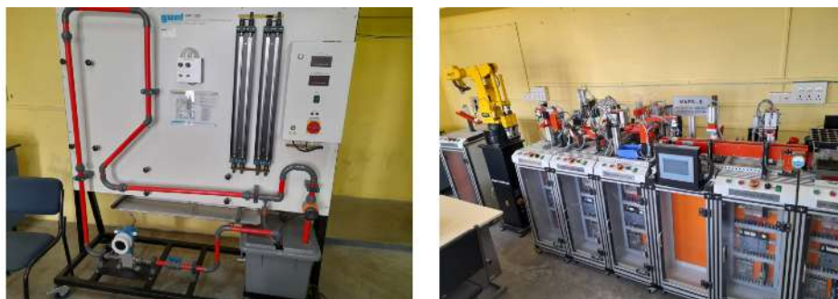
Fig. 3 Flow control trainer and PLC based robotic bottling plant.
